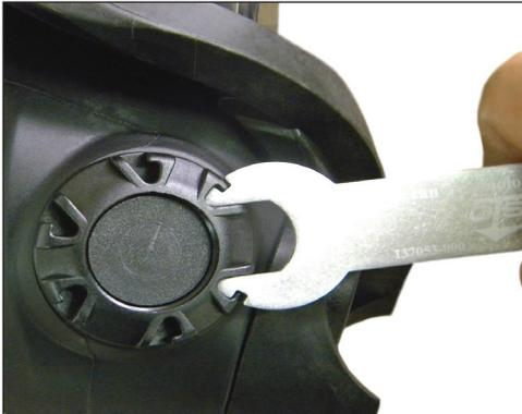
1. Locate the communications port on the right side of the mask. Using the OTS wrench<sup>1</sup> (p/n 137053-000; standard issue with Guardian FFM), unscrew the fastening nut from the plug counterclockwise and remove. The plug is then easily taken out from the inside of the mask.
