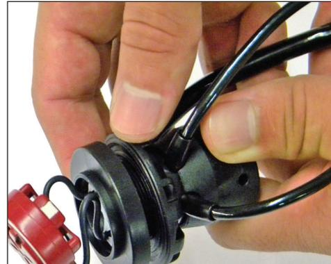
2. Loosen the captive fastening nut on the microphone/push-to-talk (PTT) module of the ear/mic assembly counterclockwise so that there is space between the fastening nut and the base of the module.
