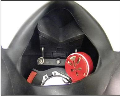
6. Once the microphone is inside the port, carefully position it within 1/4" of the right corner of the diver's lips. The ME-16R Hot-Mic® is shown above; other microphones are available (e.g., the Super Mic®, our patented\* all-depth, noise-cancelling microphone).
