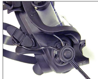
5. The fastening nut is then turned clockwise (with OTS wrench shown in step 1) until tight against the mask. Make sure the cable alignment of the OTS Ear/Mic Assembly is similar to the photo above.
