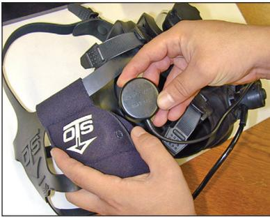
9. The EP-2 earphone is directional. With the shiny side facing toward the diver's ear, insert the earphone into the earphone holder (on each side) past the snaps with the cable positioned below the snap. Secure the snap.
