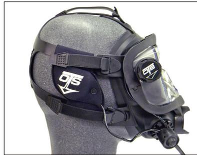
11. The completed installation of the OTS Ear/Mic Assembly. *Note: Before donning the mask, position the earphone holders as far back as possible to allow for tightening of the mask straps. Once fitted, adjust the earphone holders into position.*
