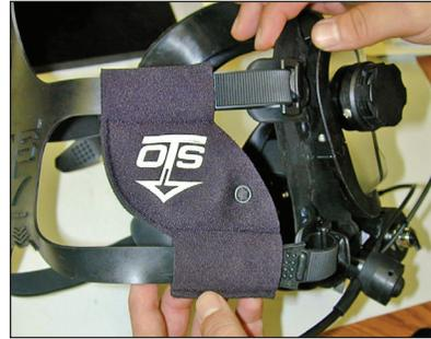
8. Insert the temple and jaw mask straps through the top and bottom slots of each earphone holder, respectively. The snaps face toward the front of the mask with the OTS logo on each earphone holder upright. Reassemble the mask straps.
