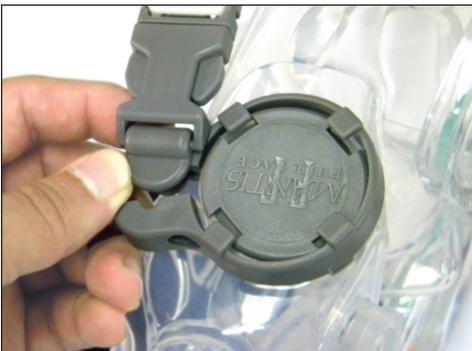
(3) Install the clamp onto the PTT assembly cap with the strap buckle attached to the clamp. Close the clamp's tabs onto the cap such that the assembly is fastened securely. Refasten the clamp screw and nut with moderate tightness.
