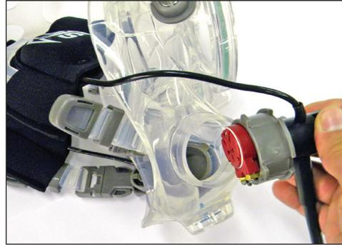
(2) Ensure the screws securing the microphone to the wires on the microphone module are tightened. The ME-16R Hot-Mic<sup>®</sup> is shown above (OTS also offers the Super Mic<sup>®</sup>, our patented\* all-depth, noise-cancelling microphone). Install the microphone module fully and evenly into the open port with the following orientation: EMMT-1, earphone cable toward the mask nose. EMMT-2, longer earphone cable toward the mask chin and shorter one toward the nose.
