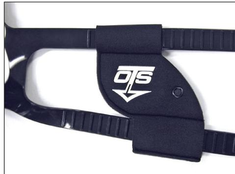
(6) Unsnap the EHA-1 earphone holder(s) from the earphone(s), and remove the earphone(s). With the snap(s) facing toward the front of the mask and the logo(s) upright, insert the mask strap(s) through the top and bottom slots of the EHA-1. Reassemble the mask strap(s) into the mask.
