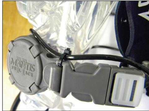
(8) EMMT-2 only: Loosely secure the left earphone cable to the buckle of the mask with the supplied tie wrap, as shown. **CAUTION:** Ensure the tie wrap does not bind the cable, so it can slide freely.
