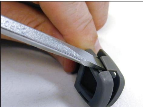
(5) Using a flathead screwdriver, separate the male and female halves of the tabs on the ends of the mask straps (right side only for the EMMT-1 or both left and right for the EMMT-2). Remove the tabs. Uninstall the straps from the mask buckles and the retainers from the straps.
