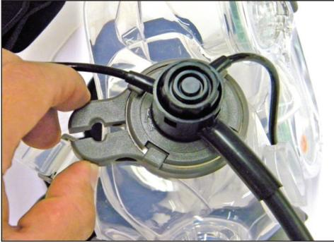
(1) Remove the screw that secures the clamp on the diver's right accessory port of the mask. Set the screw and nut aside. Open the clamp, releasing the tabs that hold the cap onto the accessory port. Remove the cap from the port.
