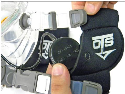
(9) The EP-2 earphone is directional. With the shiny side facing toward the diver's ear, insert the earphone(s) into the EHA-1 earphone holder(s) below the snap(s). Secure the snap(s).
