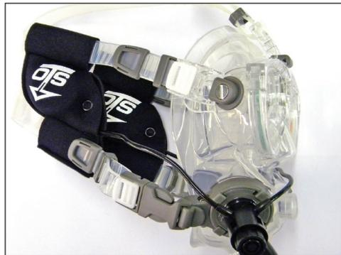
The completed installation of the EMMT-2 is shown in these next two illustrations. Note the orientation of the microphone module and the placement of the cables.
