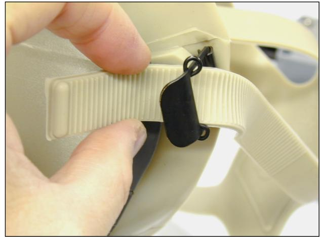
6. **Earphone installation:** Remove the upper and lower mask straps from their buckles on the left side of the mask. Find the left-side earphone holder (the one whose cable is on the left when the PTT button faces away from the diver). Feed the left mask straps through the left earphone holder such that the arrow on the OTS logo faces downward and the cable exits the holder in the forward direction. Repeat this step for the right-side earphone.
