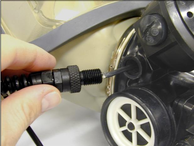
**1. Microphone installation:** Using a pair of pliers, loosen the port plug on the right side of the rebreather adapter. Unscrew and remove the plug. Insert the microphone power cable into the opening as illustrated, and twist it closed with moderate tightness.
