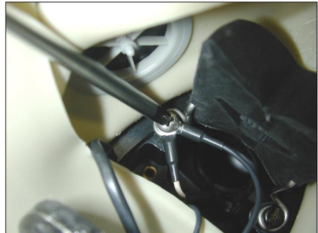
**4.** Route Screw #1 (see Step 2 illustration) through the ring lugs of the microphone's other electrical wire and the other power cable wire. Fasten the screw to the #1 position with moderate tightness.
