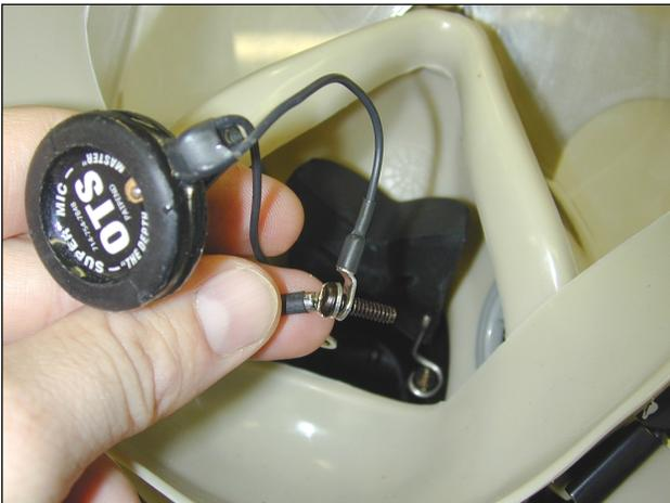
**3.** Route Screw #2 (see Step 2 illustration) through the ring lugs of the microphone's nickel-wire form, one of the power cable wires, and one of the mic's electrical wires. With the mic oriented toward the side, fasten the screw to the #2 position with moderate tightness.
