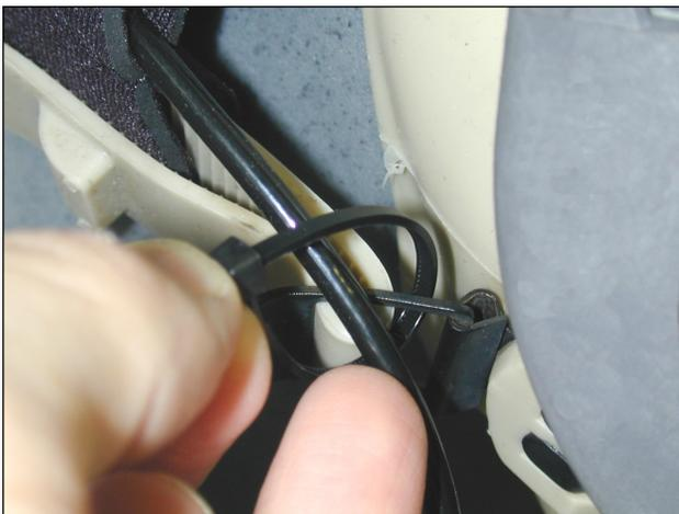
7. On both sides of the mask, secure the earphone cables to the buckles using a supplied 4-inch cable tie, as shown. Do not close the tie tightly; there should be sufficient space for the cable to move freely along the buckle. With scissors or a sharp knife, cut off the excess cable tie.
