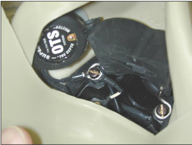
5. Make adjustments to the bending of the nickel-wire form as necessary to position the microphone as illustrated above so that it will be close to the corner of the diver's mouth. Route the wires behind the equalizing block, so they are out of the way. *The microphone installation is now complete.*
