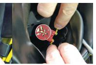
12. Position microphone to be just off diver's lips—it should not poke the diver.
