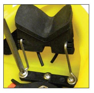
2. Attach the desired wire form to the equalizing block that creates the optimum fit for the user of the GFFM along with the appropriate pad. Align the eyelets of the new wire form assembly with the holes of the equalizer base and place one screw through the wire form and into the hole. Hand screw, then insert the remaining screw into the hole on the opposite side. FOR BEST RESULTS, ALTERNATE TIGHTENING EACH SIDE WITH THE SCREWDRIVER UNTIL EACH SCREW IS SNUG AND THE ASSEMBLY IS HELD FIRM.
