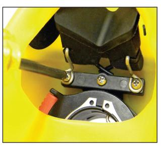
1. First, disassemble the standard equalizing wire form by removing the 2 outside screws while holding the wire form in place. DO NOT unscrew middle screw. Remove equalizing block and wire form assembly from GFFM and separate the block and pad from the original wire form.
