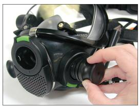
**1.** Remove the plug from the left connection port (on the left side of the mask from the diver's perspective), by pressing the colored release button on the side of the port and gently pulling out the plug.
