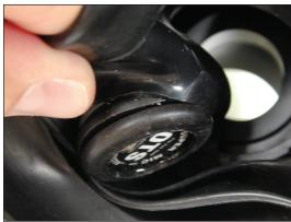
**6.** Pull the wall surrounding the opening of the oral-nasal pocket over and into the microphone housing groove. The edge of the wall must be entirely inside the groove.
