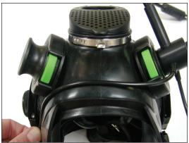
**12.** Repeat steps 9 and 10 for the right side of the mask. Then pull the right (longer) earphone cable along the groove on the bottom of the mask, as illustrated. Pull the earphone *behind* the right mask handle, and insert it into the holder. (Again, the side of the earphone marked "this side away from ear" must face outward, away from the mask.) With the cable *below* the snap, snap closed the earphone holder.
