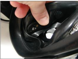
**5.** Insert the microphone housing into the opening of the oral-nasal pocket.
