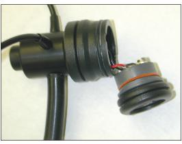
**3.** Remove the microphone housing of the EMDG-2SM from the push-to-talk (PTT) housing by pulling gently and steadily. Be careful not to damage the wires connecting them.
