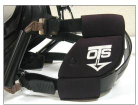
**10.** Install one of the EHA-1 earphone holders onto the mask straps, as illustrated. It should be positioned on the straps such that it will be directly over the diver's left ear. Reinstall the mask straps onto the buckles as before.
