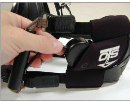
11. Identify the left earphone, which has the shorter of the two cables. Insert it *behind* the left mask handle (from which you removed the mask straps in Step 9) and into the earphone holder. The side of the earphone marked "this side away from ear" *must* face outward, away from the mask. With the cable *below* the snap, snap closed the earphone holder.
