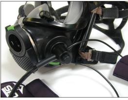
**4.** With the shorter earphone cable pointing toward the left mask strap (see the illustration), insert the PTT/microphone assembly into the open port, with the microphone element facing inward. Push the housing into the port completely, until the locking mechanism snaps to hold it securely in place.
