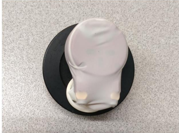
Figure 4: ME16-SL Covered in Latex Finger Cot
