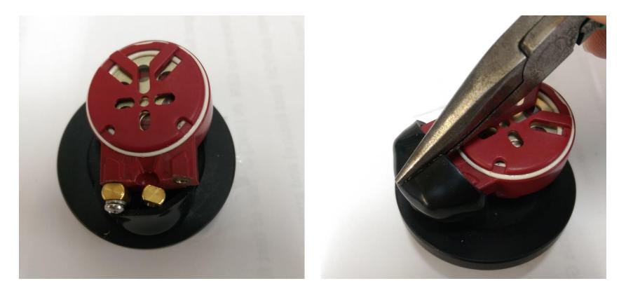
Feed boot over wire and bushings. Install screws one at a time. Pull boot over bushings with pliers.
