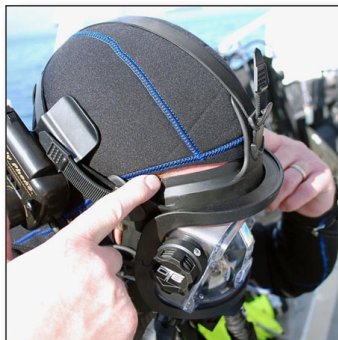
Figure 11: Fit Mask Skirt onto Skin, Not Hood
