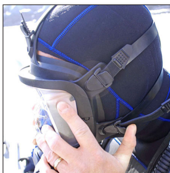
Figure 14: To Remove Mask, Grasp Bottom and Thumb Lower Buckle Tabs
