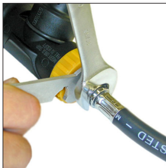
Figure 7: Fitting Hose to Regulator
