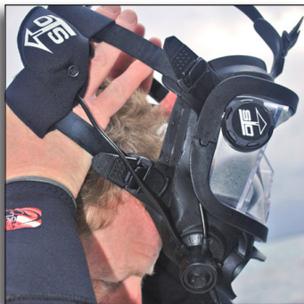
Figure 12: Open Lower Straps and Bring Over Head
