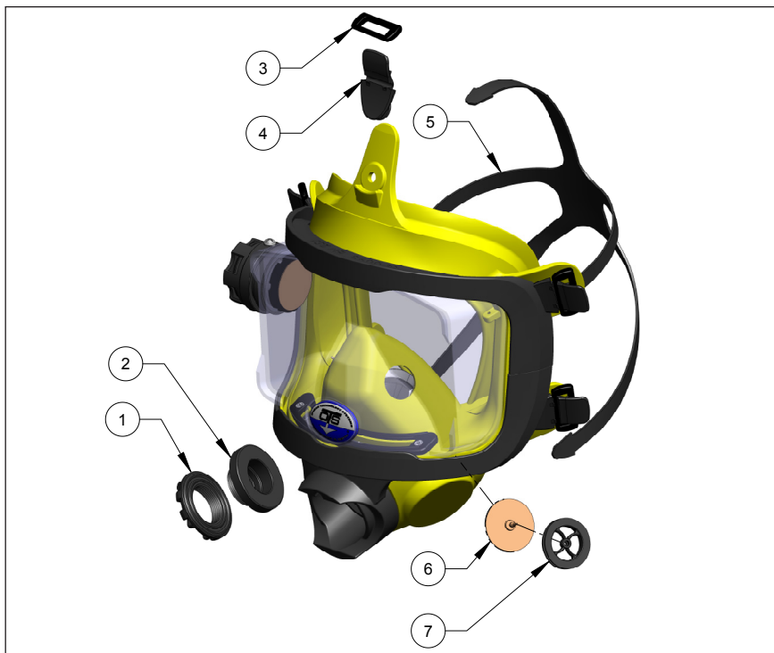
Figure 15: Guardian FFM Exploded View
